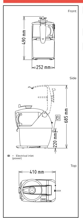
Electric Supply voltage: 600428 (DTRK45YA) 200-240 V/1N ph/50/60 Hz Electrical power max.: 1 kW **Total Watts:** 1 kW Capacity: Performance (up to): 550 kg/hour Capacity: 4.5 litres Key Information: External dimensions, 252 mm Width: External dimensions, Depth: 485 mm External dimensions, Height: 505 mm
